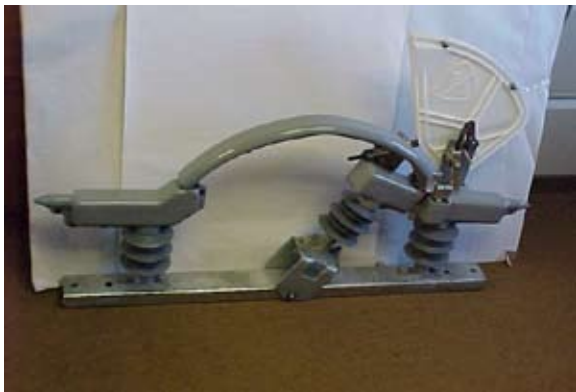
Connection Type Pole-Mounted Power Isolator RX Switch (11kv)
